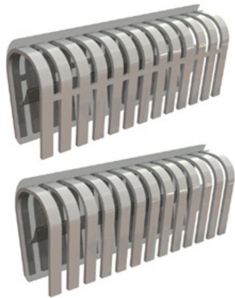
Profile with metal carrier unbroken (top) as a great grip on straight materials but is difficult to bend in curved areas as all clips are connected and made from one piece of metal. A profile with broken carrier (bottom) is easier to bend around curves as the clamps are "separated".
